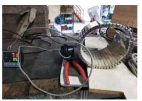
(Controller, Heater & Thermocouple)
