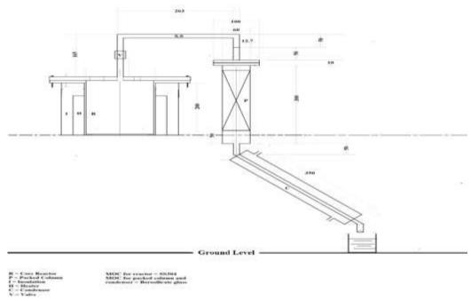
(Experimental Setup for the process)
